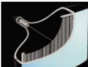
The DIAMONDTRON hybrid CRT tube incorporates a cylindrical, vertically-flat, square-cornered faceplate with an aperture grille mask design and Mitsubishi's advanced P-NX DBF electron gun which vastly improves corner focus and screen focus uniformity by reducing beam spot size.
